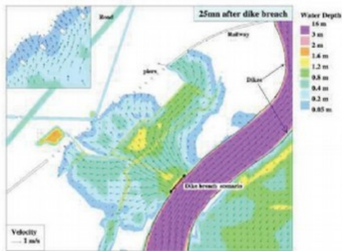
Overflow subsequent to an embankment failure
